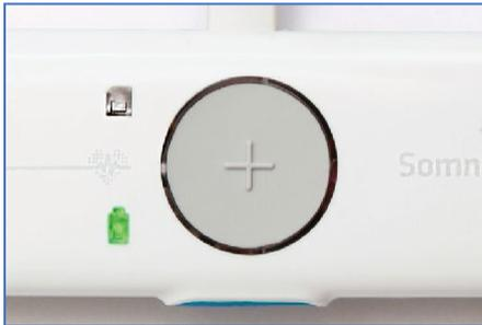
When the device is charging, the battery LED flashes in green. Once fully charged, the LED stops flashing and stays green.
