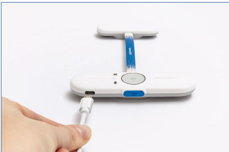
The recorder is recharged by connecting it to the USB port of a computer.
