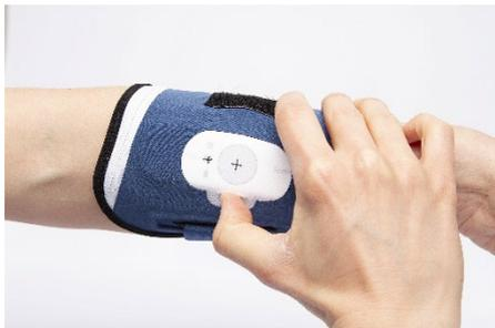
In **Manual** functioning, the recording can be stopped by pressing the ON/OFF button for more than 5 seconds.
