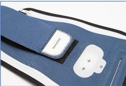
Once the device is in place in the armband and turned on, the LEDs from the device are visible through the fabric.
