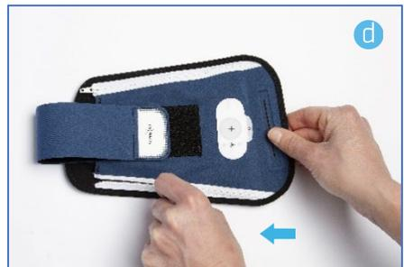
Insert the extremities of the recorder into the fixation straps. Once the device is in place, close the armband with the zippers and secure it with the central scratch strip.
