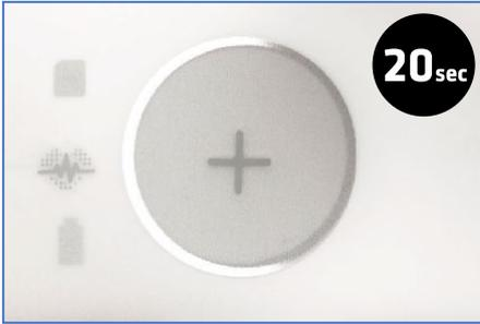
Once the calibration is complete, the recording sequence starts and the recording LED flashes according to the heart rate for 20 seconds.
