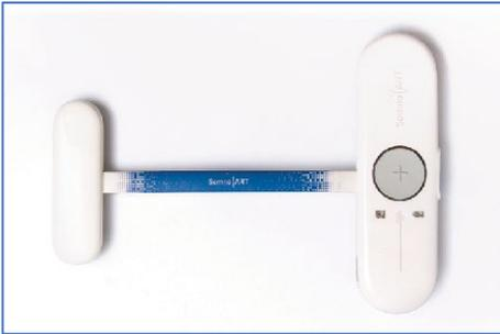
It allows to record the heart rate in beats per minute (BPM) at a frequency of 1Hz. Movements are recorded over the three axes and accumulated every second.
