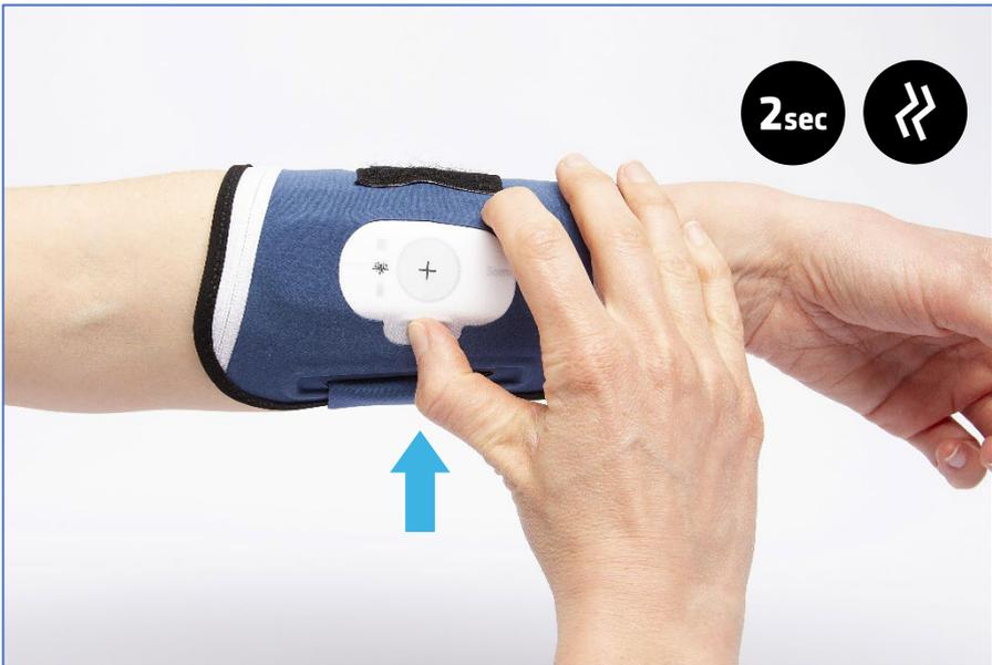
To turn the device on, press the ON/OFF button for 2 seconds. It will briefly vibrate twice and automatically display the operating state of the device for 10 seconds.
