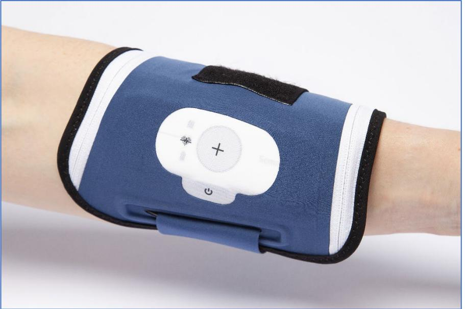
The armband must not be tightened too much, but enough so that the device will not move when the arm is pointing downwards.
