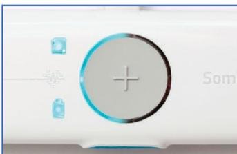
Once the device is connected, the LEDs will light up and remain blue.
