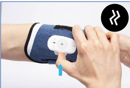
A short press on the ON/OFF button exits discreet mode during the recording. The device briefly vibrates twice, and the lights are turned on for 20 seconds, displaying the following information:
