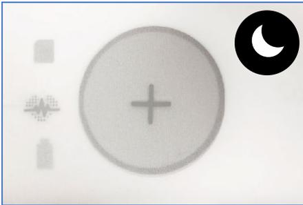
If the user does not press any button for a period of 20 consecutive seconds, the device will automatically switch to discreet mode. Even though the LEDs are not on, the device is still recording.
